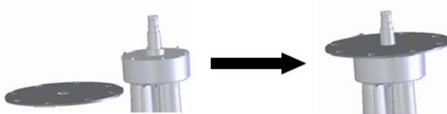
Figure 19 Inserting the Flange
