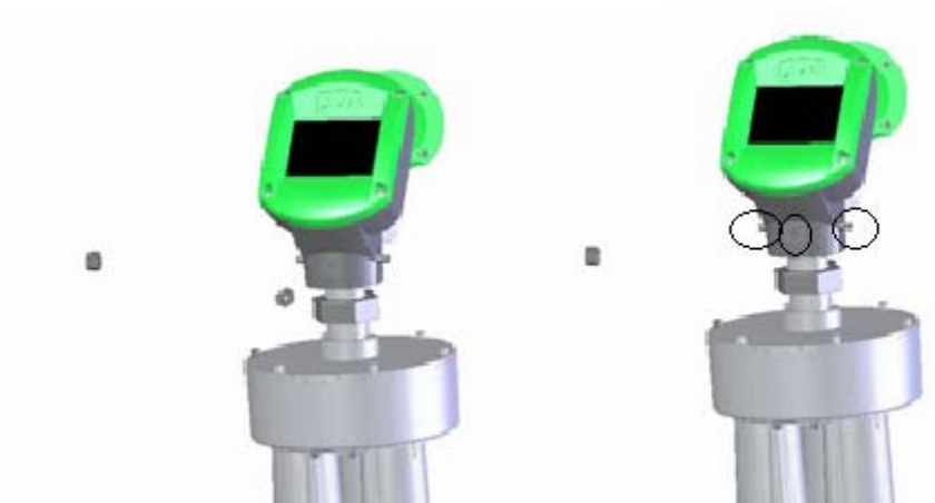
Figure 15 Removing Scanner Head Nuts and Screws
